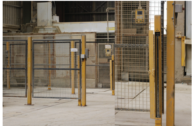
Fig 6 a&b: Use of Light Curtains at the entrance of a perimeter guarded system
