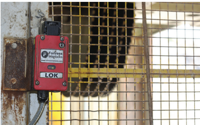
Fig 5c: Perimeter guarding and interlocking
