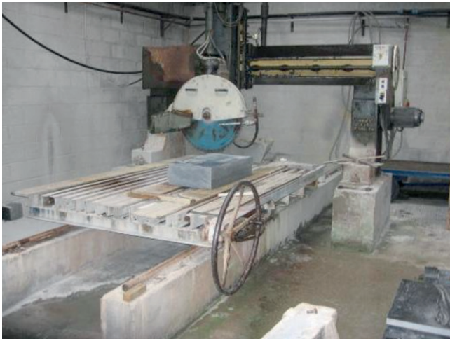
Fig 8a: Old bridge saw with controls adjacent to the saw blade
