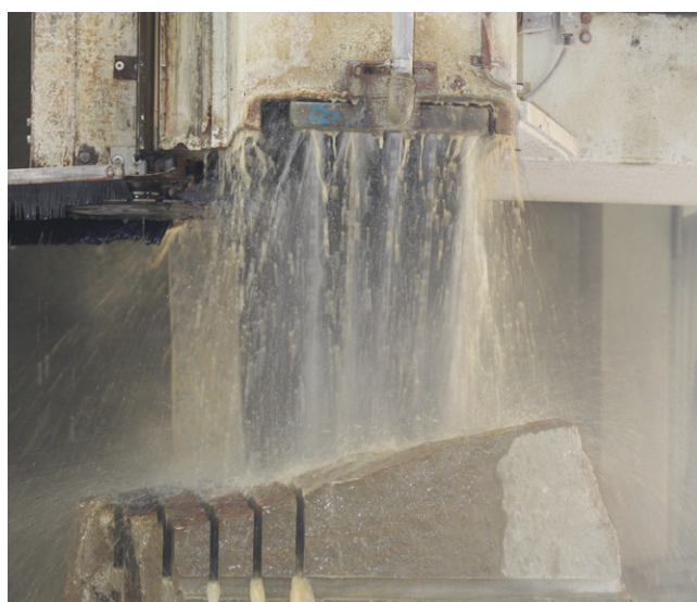
Fig 2b: Water ejected when the saw is cutting the stone block
