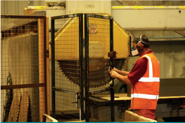
Fig 5b: Perimeter guarding and interlocking
