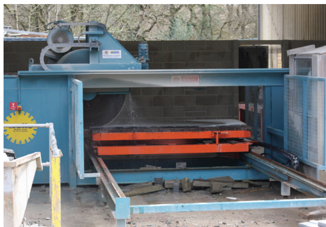
Fig 2a: Bridge saw partly protected by the framework
