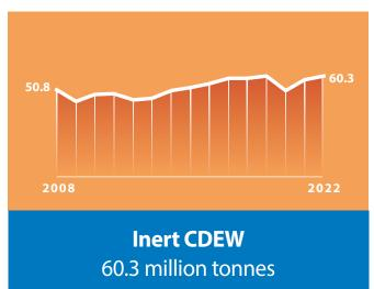
Recycled aggregates mainly originate from waste generated during construction, demolition, and excavation activities. Demolition materials are processed into marketable aggregates at either fixed recycling sites (often located on quarries) or directly at construction sites using mobile equipment. The resulting aggregates can then be used directly on-site or offsite.
